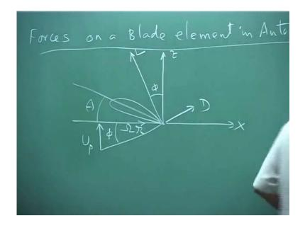
The power shaft, so note down this. Forces on, which I started, on a blade element in autorotation because here I am going to just briefly describe one section and then, we will analyze the autorotation condition and the physics associated with that. Later, you see the complexity, which actually happens in the real life.
