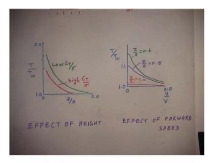
So, that is why, that particular thing is shown as a diagram, that is, T over T infinity, T is the thrust. Rotor thrust over T infinity is when it is far away from the ground and the curve actually starts from 1 to 2. Here, Z over R is the height of the rotor with respect to the ground.
