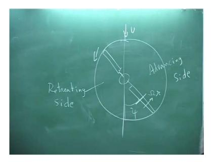
So, the forward direction I put it up. So, there is a relative wind V, which is coming towards the rotor. Now, this is also rotating, this is having omega r, so you will find... So, this is, you will have this is omega r and you have V and this is psi, that means, in this half, the relative air actually acts. That means, the rotor section experiences a larger
