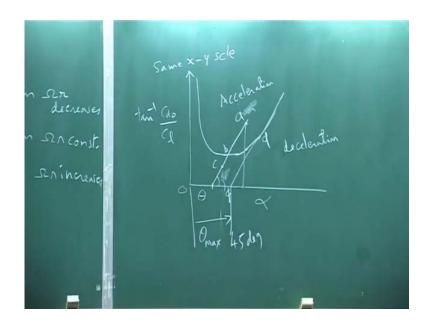
We will plot the curve of tan inverse versus alpha, but keep the axis same; axis in the sense, x-y same scale I will put it. So, you plot a same x and y scale because both are angles, this will be like this, maybe I am not drawing properly, it may go something like this.
