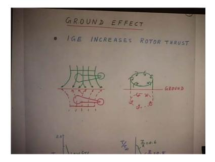
This is the ground effect; what ground effect means? Your rotor is operating close to the ground rather than far away. Because if you look at it just from what happens, the rotor inflow comes, it hits the grounder, that means, the normal velocity should go to 0 at the ground level.
