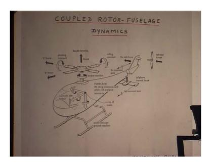
The problem which comes in coupling a rotor system to air fuselage, so this is the complete helicopter system. So, we have the rotor and of course, the fuselage is initially you can again take up a... because, it is also a long big structure; it will have its own dynamic characteristic aerodynamic whatever drag or etcetera. So, this is like and this itself can also have its own motion.
