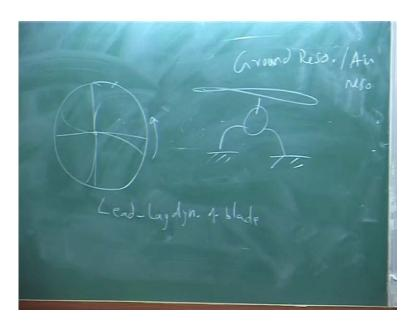
Ground resonance is the helicopter is like this it is on a ground standing in this problem what is more important of course, the fuselage can pitch and roll, but what motion couples the fuselage motion is of the blade what dynamics of the blade which couple is suppose you say this is the blade the lead lag motion lead lag dynamics of the blade.
