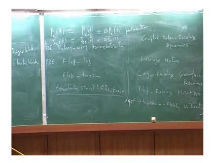
You can get into rotary-wing, aero-elasticity this is one line when I talk about rotary wing aero-elasticity. I have flap lag torsion; initially, development if you see that was not done with elastic blade rigid blade, but put flap lag combine then put flap torsion. So, flap lag problem, flap-lag flap-torsion problem, flap-lag then flap-torsion these two problems are treated initially that is one line because that you wanted to understand when the blade will go unstable etcetera.
