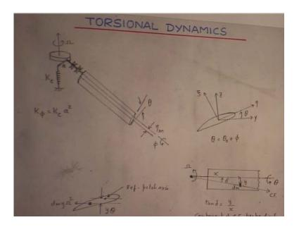
Now, let us take the next case which is the isolated torsional dynamics; but, if the little interesting; but, I will if you want I will go through the whole very simple model, please understand, very simple model. The blade is rigid blade straight and it has a pitch bearing and you have a control rod because that is the one which moves up and down to give the pitch angle change.
