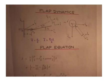
First isolated flap, isolated means only flap motion I am considering, I am not considering lead lag torsion combined because the moment I combined, I cannot show the equations. Now, you see, I have slowly, I am complicating my blade model. The earlier we had a centrally hinged and we put a spring restrained. Now, I am having an offset and a spring, this is what a real life blade is, you can represent it, equivalently offset hinged spring restrained blade model; even our blade is also similar.
