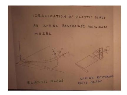
How do we analyze this problem? I will just show idealization of an elastic blade as spring restrained rigid blade model. This is your idealizing; this is the elastic blade I have shown here just for example. If you have a small element because this is how we analyze structure, you take a small element of the blade.
