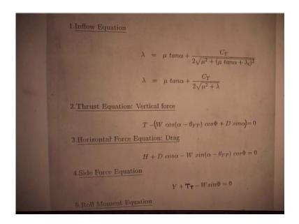
So, I said, first is inflow equation in forward flight, uniform in flow I have taken, please understand, this equation is one, then I have trust equation. When I say vertical force, this is along hub. So, this is, this is the thrust, this is T, this is my capital H, this is my, because T H Y, then you have m, x then you have m y and you have m g, all the loads at the hub.
