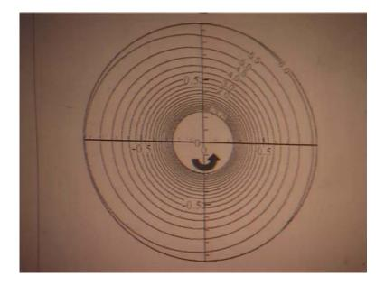
I have put the numbers here, this is 0.05,05 these are nothing, but the midpoint of the rotor. And these small numbers 2, 3, 4, 4.55, 5.6, these are effective angle of attack on the rotor disk at various radial locations because this we took it as 0.23 as the hub for a
