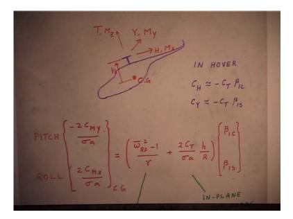
Moment about the hub center, because these are all for controls, flying, you need to know that value. You assume that the C G is here rotor hub is at a height h just I am putting it right on shaft, it need not be straight on shaft, it can be anywhere a little displaced those things, will come when you do the actual problem. Now, you have a hub H longitudinal force M x which is the roll moment. Similarly, you have y which is the
