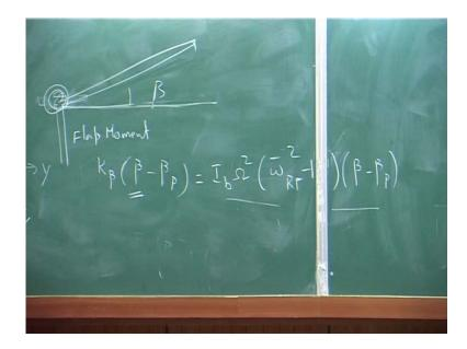
Now, let us write this quantity that is the moment, flap moment. I will write it flap moment I b omega square omega bar R F square minus 1 into beta minus beta p. So, I am converting, the spring stiffness directly in terms of flap frequency, rotating flap frequency. This is a modification just because you know that what is K beta. Now, usineg this, I will go get my moment, because this is my psi. So, this angle is also psi I take along x and y what is the moment.
