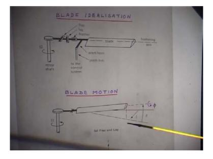
Because if you remember right at the beginning of the course we mentioned the blade is attached to the hub and then a if it is articulated, you have a flap hinge and you have a lead-lag hinge and you have a pitch bearing. And in the case of a hingeless, you do not have any hinge, but you have a pitch bearing, because you need to change the pitch angle of the blade cyclically, as it goes around.
