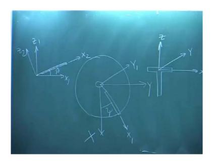
And the blade can be inclined, flapped, it can do anything it wants. But my motion is describe in this plane. This is my reference plane, which is same as what I do in the fuselage, because this is attached to the fuselage, so once you decide this frame, you can say this is parallel to the c g frame also if you want, but it can be little different also.
