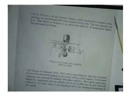
Now, I will give, there are lot of pictures, different groups of people and this is in Austria. Lieutenant Petroczy and von Karman constructed a tethered contra rotating co-axial helicopter with three engines of 60 hp each, the rotor diameter was 6 meters. Vehicle was designed as a platform, observation platform. Even now people talk about observation platforms, but it made several flights, but had control problems.
