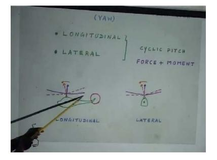
But the problem is when you tilt the rotor, this is the horizontal thing, I tilt it, so my thrust is here. Initially, the CG is right here, is coming down and holding it. Now, what happen because of the tilt? It has gone; I am going to get a moment about the CG. Now, the moment also it will come. Now, if you do not balance the moment properly, then you will have, you cannot control the rhythm. But how the moment is balanced in the helicopter?
