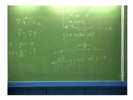
Now, you are considering formation of wave over a flat surface. This is my mean unreformed datum and in this direction we are plotting z. This is wave, let us say the wave is forming (Refer Slide Time: 15:15). Basically, we have this surface at z equal to minus h and that is at the bottom, what do we expect there? There should not be any normal component of velocity. Since, we are doing in this analysis it will allow a tangential component but, no normal component.
