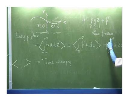
If I look at a wavy interface, the energy flux would be created because there is a pressure excursion, so pressure is varying as you go along in the x direction. So, what we could do? If we keep our attention fix at a particular say perfectly harmonic component and this is your x equal to 0.
