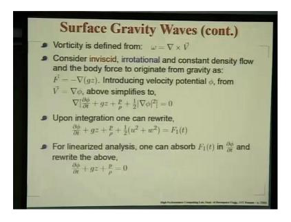
This term comes from the del v del t term, this comes from the body force term, this is the pressure gradient term and this is one path of the connective actualization which survive after irrotational approximate (Refer Slide Time: 24:20).
