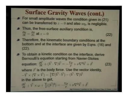
As I told you that we began this analysis, saying we will be doing some kind of a linearization looking at small amplitude waves. So what we would be doing is, we will be making some additional simplification at this condition that I am applying at the deform interface would be reflected back on the mean interface; that is what we are saying that condition will be transfer to z equal to 0.
