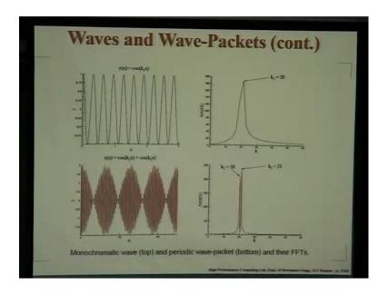
First of all, let us try to distinguish what we get by looking at waves and wave packets. So on top what you are seeing is a simple harmonic wave and which is characterized by let us say this wave number that we have plotted here for k 1equal to 20. This is the way the signal varies with phase that cause k 0, k 1 x is plotted here.
