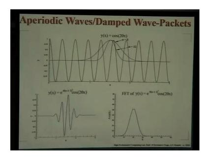
So, there is another way signals are quite often transmitted. Those are when this signal is embedded in amplitude envelope, which renders its aperiodic nature. So what happens here, we have the basic signal for 20 x let us say; then, we modulate its amplitude by this Gaussian Function, then what happens is the signal information that you are carrying still corresponds to 20 x, but it is amplitude decay.
