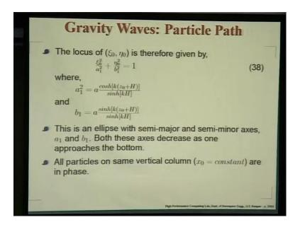
If I just simply find sin square kx0 on this, so that is why we have eliminated equilibrium coordinate and t and that will be all given in terms of z0 and A as amplitude of the wave. You can very clearly see this defines an ellipse; the ellipse is given by this semi-major and semi-minor axis. You notice that as you go towards the bottom of the liquid, z0 is going to progressively go towards minus H.
