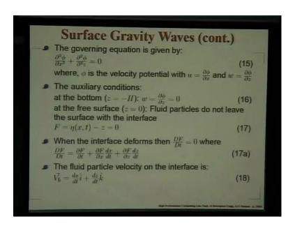
Now, what do we get? The governing equation here comes from the mass conservation equation that is delta at v equal to 0 and where v is essentially for rotational flow. We can write it as a gradient of a potential pi, so it is here and you get equation 15. The Laplacian of 5 in that exert plane is going to be 0 and the velocity as I noted here, the components are given as the x component del phi del x and the z component is del phi del x (Refer Slide Time: 14:42).
