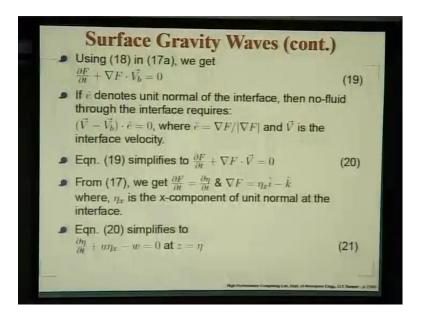
Now, if I define e cap as the unit normal on the interface then, the condition that we have said that there is no fluid through. So, what will happen is the velocity of this fluid particle that is vb and v is the velocity of the interface they would essentially be same. So, there is no discontinuity. So, that means the dot product of that with respect to e cap equal to 0, where of course, if F defines the interface e cap is nothing but, gradient of f divided by the modulus of that gradient.
