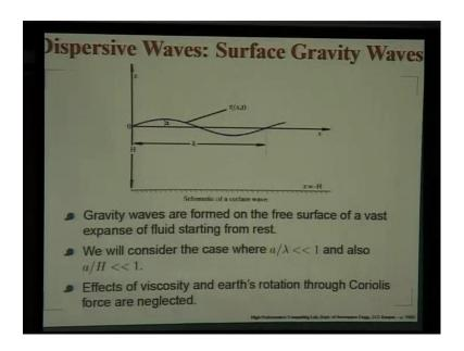
Now, let us get into some detailed look into one such mechanical waves, that is created over a vast expanse of fluid and you have a fluid at rest, then you just give a kind of a disturbance on the surface. So the surface will be deflected. Let us say, we have tried to create a single harmonic wave here, whose wave length is given by lambda and this surface wave that we are creating on the surface is firming over a layer of liquid of height h and the deflected control is given by eta x and t.
