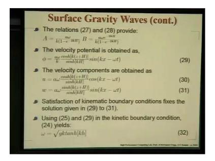
Having obtained the velocity potential you can calculate the velocity by differentiating it with respect to x will give you u, differentiate this with respect to z, you will get w and what is left? That is of course kinetic condition; the kinetic condition would come about I think, I have misguided you that is what happens then you are in a rush sorry this is not this is the kinetic condition and I mix it up for you sorry for that mistake let me just work out how do I get that...
