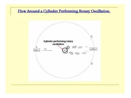
Now, show you an example of a problem; this appears very simple. What you have is basically a cylinder, and this cylinder is performing some kind of a oscillation; it is going back and forth. So, that is what we call by rotary oscillation; it is not just simple rotation, it is doing a rotary oscillation. So, what happens? Half the cycle part of the flow on one surface will be opposing the convection direction. So, suppose, let us say, the flow is going from left to right here.
