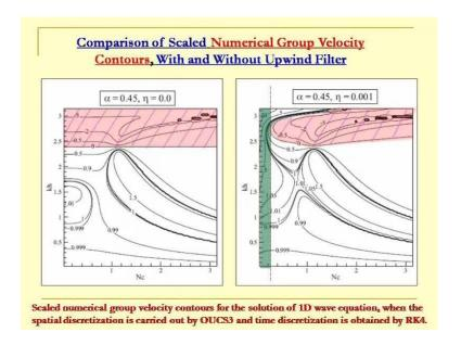
However, what was intended in doing this exercise was is given in this figure. If we used a central filter, then we identified a region of q waves here, shown by this shaded area; so, this is your v g n by c equal to 0 line.
