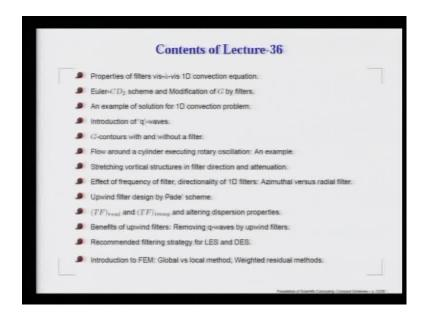
Lecture 36, and we continue our discussion on properties of filters with the help of 1D convection equation. We pick up a basically unstable Euler-CD 2 scheme and we design a transfer function in such a way, that we can modify the numerical amplification factor G with the help of this and solve this problem in a perfectly neutrally stable manner.
