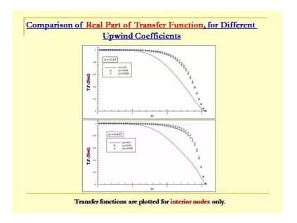
Now, the previous case was for a eta equal to 0.001 and alpha was a 0.45 here. We are basically seeing the effect of real path for different upwind coefficients and you can see its its got quite a bit of a control for us, because if I take eta equal to 0.01, I can see the filtering operations start from a rather a moderate value of k h of one itself; whereas, if I keep reducing the value of eta, the filtering gets delayed to higher k, right? So, this is what you see at 0.45, alpha equal to 0.45
