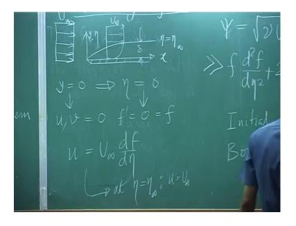
So, the domain that we will have to be looking at as I told you the shear layer forms like this. What we do is this delta, the boundary layer thickness that we talk about has been stretched out by the eta coordinate. That was the whole thing that we telescope it to a larger distance. Then what happens is we have two conditions here; we do not have any idea of any other condition that we could generate from this.
