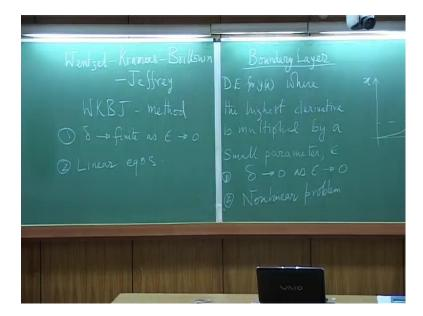
The second difference of course, is the very relevant one that this only works for linear equations. You can study linear equations. Well, but here boundary layer theory is little more versatile; it can also tackle non-linear problems. In fact, you noted that the boundary layer equation that we solved was a non-linear PDE and we could tackle it with quite ease.
