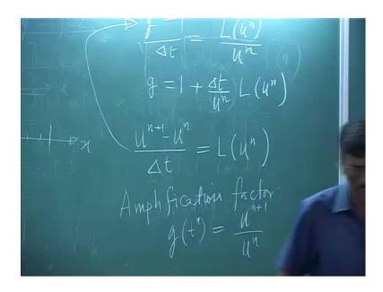
Say, give a simple example, if I have a simple equation like this with a first order time derivative written here. What we could do is we could approximate this first derivative in the left end side by its approximation at n plus 1th level. As I have told you I could do it in the simplest possible way would be to relate it to the events that had occurred at just the immediate predecessor time.
