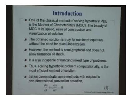
Here, we have characteristics which are real and we would like to basically make some introductory comments. One of the classical methods of solving hyperbolic PDE is what is called as method of characteristics. So, there actually we track the solution along this characteristics and it is a very elegant method, because of its speed and because of the ease with which you can really construct the solution. It is also provides you a glimpse of the way the solution actually propagates.
