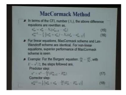
This is in the Mac Cormack scheme where you do it in 2 steps and in terms of the CFL number you could write down the algorithm in terms of equation 15 and 16. It is easy to show that if I have a linear equation that this Mac Cormack scheme and Lax-Wendroff scheme; they are basically identical. It is only for non-linear equation that you derive more benefit from Mac Cormack.
