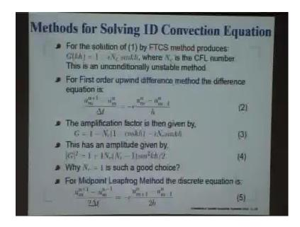
One of the simplest examples of hyperbolic equation is this 1D convection equation that we have seen. Let me just simply go through and tell you we already know that FTCS method, this is the forward in time central space method. We find that G amplification factor is given by this, where N c is basically the CFL number which you have familiar with; we are not talking about it because this is a conditionally unstable method, it is going to be of any use at all.
