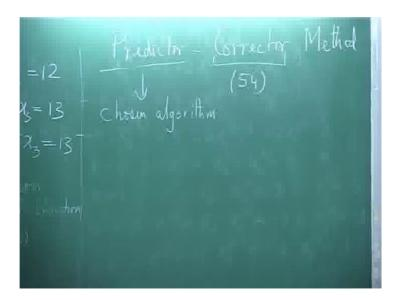
You have a predictor method. You predict it the way any algorithm that you choose. Let say, it could be Jacobi, could be Gauss-Seidel - you would do that and then you obtain that. This u over bar l plus 1 is output of the predictor stage.
