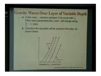
So, what happens is in this case, omega remain constant if we move with the variable Vg. Another wave parameter like k and c, they will all change with x. The ray path now will not necessarily be straight, they will be all curved. What we are seeing then this curve path corresponds to omega equal to constant, whereas the ray path - these are the path which defines a group velocity by its slope. So, you can see it keeps changing with the position.
