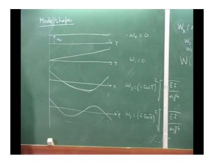
So, this is W, so this is my x, so this is constant this is W 0 that is the first mode, frequency omega 0 is 0. And the second one, I can take it like this it is a rotation c 1 x, and this is also omega 1 is 0, when I go to the third one, how it will vibrating it will vibrating this is at 1 this is the length 1, maybe I should plot it. And for this the frequency will be 1.506 pi wholes square E I over m 1 4, because I have taken 1.506 substitute that beta, and get the omega square.
