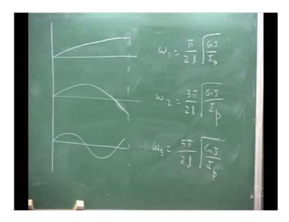
So, this is the shape and this is the what you get is now you plot, the mode shape you have sin wave this is 1, and the second one will be like this and the third. So, you will have omega 1 is pi over 2 l root of G J by I p, omega 2 3 pi over 2 l root of G J over I p, and omega three is 5 pi over 2 l root of G J over I p. So, this is for the torsion problem, so you have the complete I would say simplified problem solution, which we know how to solve now.
