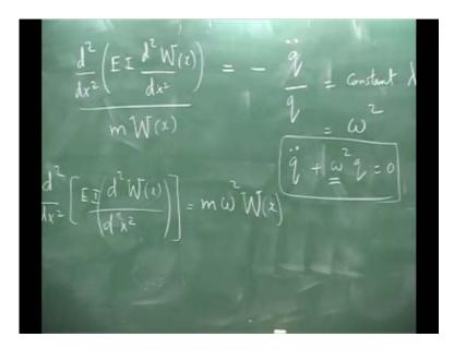
So, free vibration of a bending problem, because I just want to indicate one thing and then, free vibration of a beam. You write it, z of x t is 0, so I will have my equation E I del square W plus m is 0, of course boundary condition will keep them at there, later we
