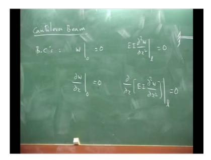
So, the interesting part is, for a cantilever beam, boundary conditions that will become displacement will be 0 that is, W at 0 is 0, delta W by delta x at 0 is 0, the slope is here. I have put restricted and then, you will have E I del square W by delta x square at 1, this is 0 and delta over delta x of E I del square W by delta x square at 1, 0. So, you see, these are the boundary condition for a cantilever beam, these are the boundary condition for a beam with the, this is one.
