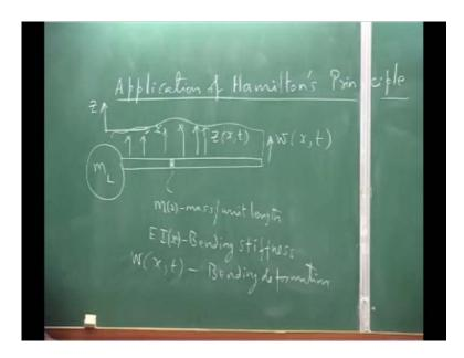
We call it application of Hamiltonian's principle, but what we will do is, we will formulate the equations for a beam like structure under bending deformation. Then we will use the same principle equation for again a torsion problem, that way you have bending torsion of beam like structure derived, which we will be using it for the later aero elastic analysis. Now, let us take, the wing is represented by a beam, I am not put it as a cantilever beam or anything like that.
