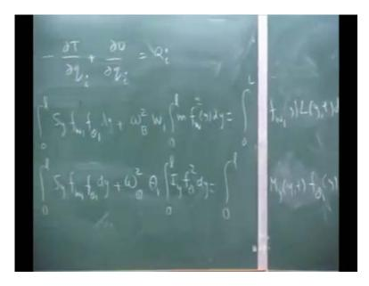
Now, you can write your equation of motion, substitute in Langrage's equation and then, get the equations, because you know Langrage's equation. Now, let me erase this clear, because Langrage's equation is d over d t of delta T by delta q dot then, because here T is not a function of q, because only q dot it is there, that is why the term will go off
