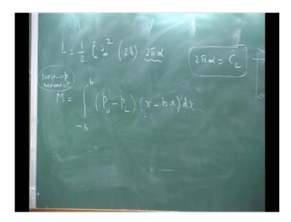
You got your put a lift for unit length by this expression, lift is half rho infinity u infinity square this is the dynamic pressure, card is 2 b and then c l, c l is 2 pi alpha this 1 infinitely is alpha c l lift coefficient. This you call it as which is directly on all time into two types pi, so this is the theoretical value. Now, if you want moment again it is minus b to plus b, you take it as p u minus p lower and moment about what point you are taking, because I put a diagram like this.
