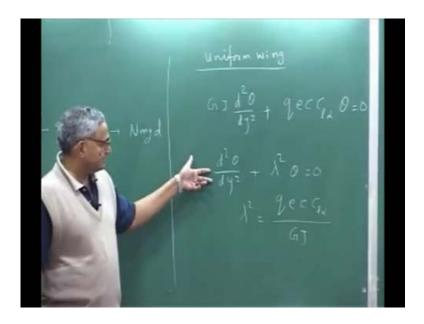
First let us say, it is a uniform wing when I that means, G J e c C l alpha, they are all constant and I look at the only the homogeneous part of the differential equation. That is not the particular solution, because I want to see how the homogeneous solution changes, what is the form of the solution and what condition it will be towards the divergence speed. Because, the key parameter is the q, which is the dynamic pressure, which is half rho U square, which can vary with forward speed.
