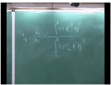
So, I am going to write my divergence speed as or q D becomes k 1 1 by B 1 1, which is nothing but, integral 0 to 1, G J phi prime square d y over integral 0 to 1, e c C l alpha phi 1 square d y. That is very simple, I got just divergence speed and I can have, but this is with only one mode approximation please understand, if I have two mode approximation then I will have 2 by 2. Then I have to solve for the Eigen values, this just the single mode approximation.
