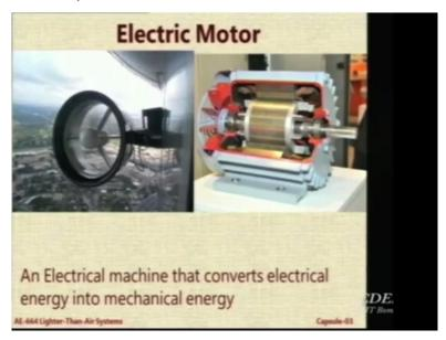
Now let us come to the electrical motors. So electrical motors essentially are it is a machine that converts electrical energy into mechanical energy. And some pictures. So first picture on the left hand side shows the electrical motor installed on the airship gondola. And the one on the right is a cutaway view which shows the winding and the magnets and you all know how it works.
