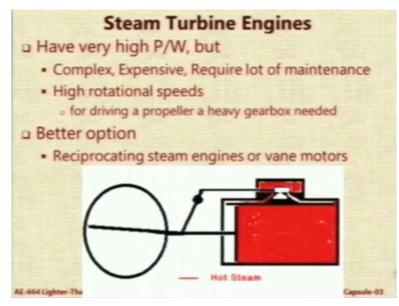
So steam turbine engines very high power to weight ratio and that is the principal attraction. The power available versus the weight of the system is very high, but they are not very straightforward to operate. They are complex, expensive and require a lot of maintenance. Secondly you need very high rpm's. Therefore, you need a very heavy gearbox because the engine will produce high rpm and to reduce it down to the propeller rpm you need to protect the gearbox.
