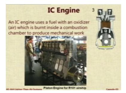
Let us go to IC engines which are very common. So, essentially an IC engine is one that uses an oxidizer which is mostly air and that is combusted inside a commercial chamber and that produces the required energy for the mechanical work. (Video Starts: 09:40) So, you can see the functioning of the IC engine as shown here in this small video. So you can see that the piston gets compressed and then there is an explosion.
