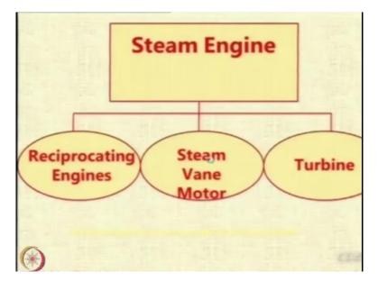
And inside engines also there are various subsystems. What we saw just now is the reciprocating engine. So, steam is used for a reciprocating piston. You can also have vane motors where there are some cup like things which move, rotate because of the flow of high speed steam. You can also put a turbine and make a turbine move by impinging steam into it. All of them have their pluses and minuses.
