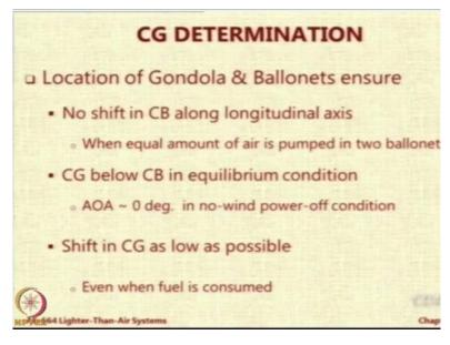
And location of the fuel tank should be such that when even when fuel is consumed, the CG will shift. It will go up because fuel is on the bottom and the fuel is being consumed that should not be too much. All of these are going to affect the trim condition of the airship.
