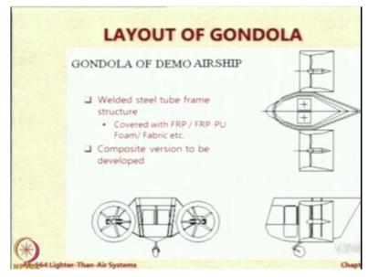
So, the gondola was, this is a demo airship. It has to be light, it has to be made quickly. So, either welded steel tube framework with FRP-PU Foam, etc., or a composite version. This was a simple gondola that we designed. So you can see there are two ducted motors, one on each side, and just a small gondola. We have given two seats. But actually it can take only one pilot.
