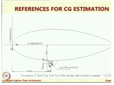
So, there are some references used. For example, there is x, y, z reference at the nose. Then there is a reference for the center of gravity of the gondola, CG, etc.
