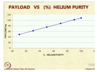
What happens with helium purity? Notice that when the purity of helium is 100% if the payload is 115 kg, it shoots down to only 50 kg if the purity of 91%. So, there is a linearly reducing effect of helium purity. This is because the buoyant lift becomes less straightaway. The impurity which will be air will not only reduce the buoyancy, but also increase the weight.
