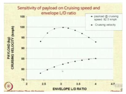
Similarly, we plotted out the l/d ratio. How does l/d ratio because as you know l/d ratio is going to affect the aerodynamics. So, there is a peak. It is a very interesting result. It tells you that this l/d ratio of around 3 or 3.05 is actually the peak. This is the GNVR shape. So, you make it less than this and the payload decreases. You make it more than this, the payload decreases.
