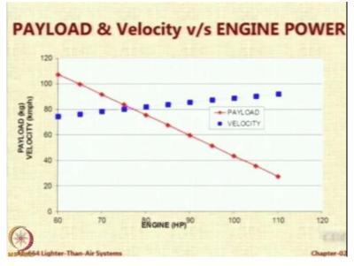
Then payload and velocity versus engine power. So, on the y axis you have either payload in kg which is the red line or velocity in kmph which is the blue line. On the bottom on the x axis, you have the engine. So, you notice that as the payload decreases, the engine horsepower follow suit and as the cruise as the engine power increases you can get slightly more cruise speed also, blue line goes up.
