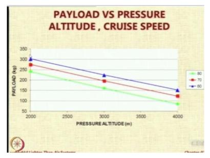
Similarly, effect of speed. So speeds of 80, 70, 60 for a given pressure altitude, you have to go vertically on the lines. So, you see there is a small change. There is a change, but a small change. So, 250 kg payload is available with 80 kilometres per hour, maybe 275 with 70, maybe 300 with 60, So, 25 kg more for 10 kilometers per hour difference, but the loss in the pressure because of pressure altitude is much larger.
