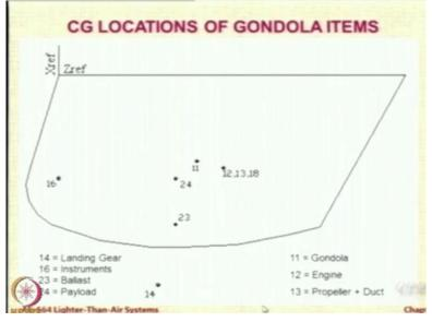
Gondola has got so many items. Instruments, landing gear, ballast, payload; all of them where they will be and then find the center of gravity.
