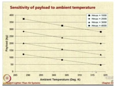
This information I have already given you in the previous graph. Now, I am just plotting it reverse. I am plotting the same data for various maximum altitudes. So, all of them decrease linearly. So 50 kg payload becomes 120 kg payload if the temperature is reduced. That means if you operate in a cold environment, you can carry more payload.
