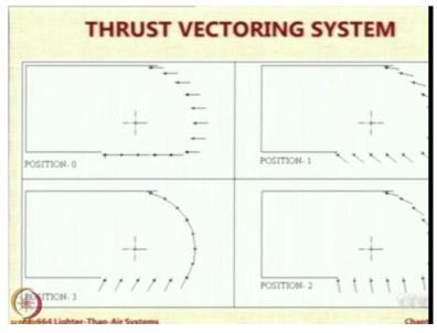
Then we thought let us go for some thrust vectoring system. So our concept was to have a load type system so that you can deflect a series of flat plates, which can deflect the slip stream rather than tilting the engine or tilting the nozzle. We said we will just tilt the slipstream by flat surface. We could never get a chance to build this, but this was one project and this is still available as a project for someone who is interested in developing a thrust vectoring system.
