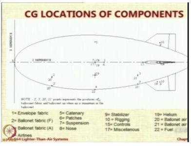
And then for each component with little bit detailed calculations, we made a 3D model and got the lightly CG location. For example, if you see number 5, number 5 is a catenary which are basically ropes that go inside the ship to hold the gondola or transfer the load on the top. Then number 10 is rigging. Number 9 is the stabilizer, 15 is the controls, 4 is the air lines or the
