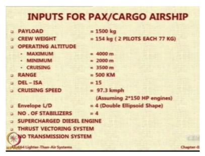
So what are the inputs for it. The inputs were same as that for the demo airship but for the payload and the envelope shape. So for this, we did not want to go for l/d of 3 GNVR shape. We went for what is called as a double ellipsoid shape, 2 ellipsoids.
