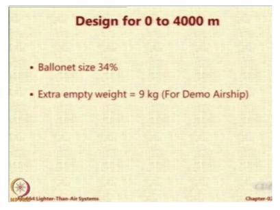
Then we wanted to know suppose we make an airship which goes from 0 to 4000 delta H, so we found that instead of 20% it is 34% ballonet size. So, the inflation fraction will reduce from around 80 to 66. And because of that you have 9 kg more weight. So, that means the payload capacity which was 77 kg will become further less if you have a larger ballonet.
