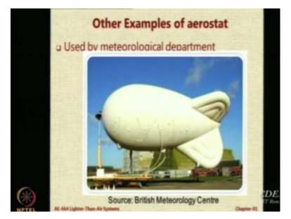
Another example is for collecting the meteorological data, so for that small aerostats like this can be sent up or can be stationed at a particular place for a long time you can collect data regarding the weather, atmospheric properties and many other parameters which are difficult to calculate. For example, if someone wants to do a study about pollution happening because of a chimney in one particular area.
