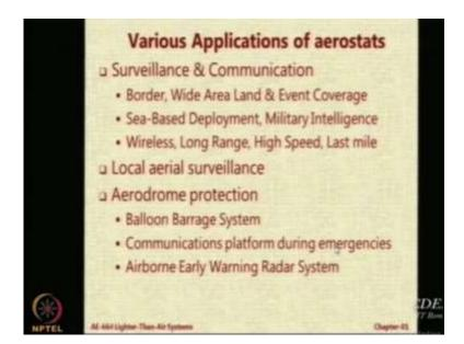
Let us see the applications of aerostats again. These applications are ones which have already been done, so surveillance and communication you can use it for surveillance at the border, surveillance to give huge coverage. the Indian air force. For example, has installed aerostats for aerial surveillance, they are typically installed around 50 to 100 kilometers inside our territory and they can give a visual coverage of around 350 kilometers.
