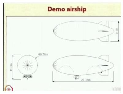
Now, let us look at some more details. So, here is the 3-view diagram of the demo airship that we got. You will notice that the maximum height is 11 meters. Diameter of the envelope itself is around 9 meters, 8.78 meters and the length is 26.78 meters. What does it carry? Only one passenger and that is a pilot. So what had gone wrong? Why do we have to have 27 meter length and you know 11 meter height just to carry pilot itself and the pilot.
