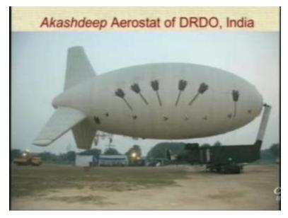
This is one of the recent aerostats developed by the same laboratory. And this photograph was taken at the aero India show. So you can see that there is very neat winching and mooring system developed instantly by LnT in Powai. And then you have this envelope and here you can see the payload is mounted in this case directly onto the envelope ok. So let see there is very interesting news..
