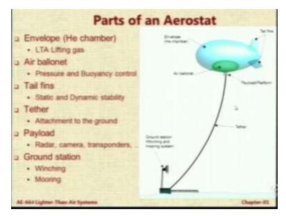
Alright let us look at what are the key parts of the aerostat. So the first and most important part obviously is the envelope. Here we say the helium chamber because we are assuming that helium will be used but it could also contain hydrogen or any other lifting gas. So it is basically the one that contains the liquid gas so it is nothing but the container, it is nothing but the envelope to carry a given volume of gas.
