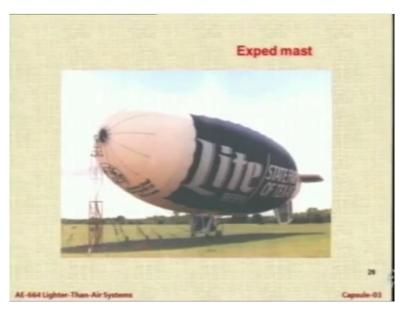
And then we have this exped mast which is a truss type structure. A truss type structure which also is then attached to the ground. This is also one more type of mast structure which is used for attaching the airships. And also what you see in the front of the airship is some kind of a disc where which the mast is attached and then you see these members. So what do you call them?
