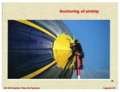
This is how on guyed mast the airship is anchored. Even today there is the mast man one particular position who basically receives the airship and attaches it to the to the mast. Now, we have done some work in our laboratory on mooring masts with the help of students like you mostly undergraduate students. So, mast have been made, designed and fabricated both for indoor air ships as well as outdoor air ships. So, now I want to showcase some of the work that we have done.
