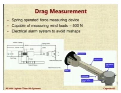
And then the system that was actually fabricated for drag measurement was much simpler than what was given in the previous. This is the improved design. In this improved design, you can see that there is a small enclosed drag measuring device.
