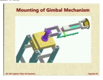
This is another view of that. So his design was to go for a structure consisting of an assembly of 4 rectangular channels which are commercially available in the market joining them by either welding or by bolting and creating this system. And then there was an indicator here which gave indication of the force acting which could be calibrated. And the idea was that when this is going to touch some number, there will be a contact and the alarm will go off.
