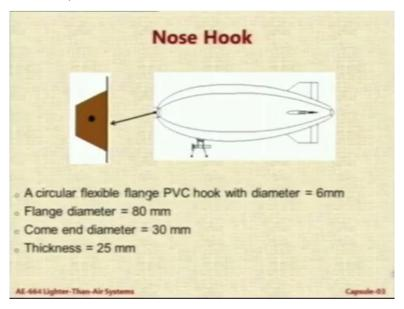
Now, nose hook is very important because you need to have some kind of a contact between the flexible envelope and the rigid mast. So, there are many schemes possible as we will see. In this particular scheme, this airship was just under 5 meters long, it is around 15 feet in length. So, for this particular airship and we were very critical here about the weight because it did not have too much of spare lifting capacity.
