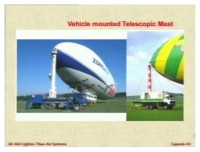
And then we have these modern vehicle mounted telescopic masts. So on your left you see the blue colored truck. It is a hydraulic mast and it can actually fold and go on the truck. The truck can move with the mast in the unfolded condition. So, the idea is that if you launch it from a
