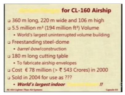
Now let us learn a little bit more about it. Look at the dimensions of this hangar. The length is 360 meters. The height is 106 meters, it is more than 100 meters high and the width is 220 meters. So at 5.5 million meter cube, this is the world's largest uninterrupted volume building. And the next largest building is the factory of building at Everett which makes the final assembly but that is occupied building.
