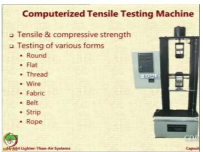
So finally, we will look at some work that we have done in our lab on characterizing these fabrics and for that some machines have been procured and installed in the LTA systems lab. So, I will just showcase to you these machines one by one. This is a machine that we have for dedicated machine, special purpose machine for testing the strength of ropes or fabrics. So, in the current configuration that you see the jaw that has been put, this is the jaw of the machine.
