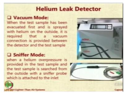
Then the next equipment which I want to showcase is a very special equipment is the Helium leak detector. So, as you know helium is one of our preferred LTA gases and leakage of helium can be disastrous from the point of view of cost and operational efficiency. So, let us say one of you makes a small airship or envelope for aerostat and now you have fabricated it, but how do we test it for leakages?
