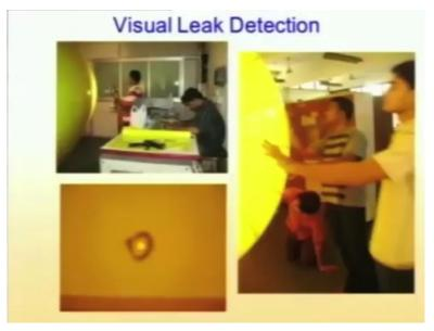
We use what is called as visual leak detection method. So what we do is on one side of the envelope we illuminate with the table lamp. you can see Vishal is holding a hand held table lamp, made the room dark. On one side put a table lamp or a big illuminating bulb. On the other side the whole team starts looking. Now light is something that can come outside the hole. If there is a pinhole, you will see star like illumination points.
