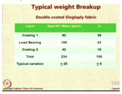
Here is an example. This slide is only meant to give you some kind of a mental picture of the weights. How much does it weigh? So, a typical load bearing member would be around 100 grams per square meter 100 GSM. You coat it on outside and inside. There will be a difference in the coating required. The coating that is required for providing the environmental protection weighs more than the coating that is required for gas retention.
