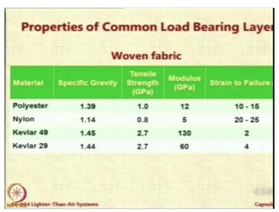
If you can look at the load bearing layer, these are 4 candidates for the load bearing layer. Polyester fabric is very commonly used including for shirting and suiting. The same fabric can also be used for base load carrying member of the fabric. So, you can see that it has a tensile
