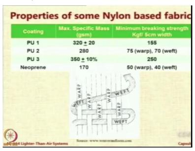
Now, here is a picture which explains to you what is meant by the warp direction and what it meant by the weft direction. In a typical woven fabric we use long longitudinal fabrics and then you weave them with lateral fabrics and the lateral fabrics normally are continuous which go along the width. So they are called as the weft which are used by the weavers and the warp is along the length.
