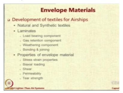
Now, the envelope materials have come over the years by a large amount of R & D in textiles for airships. So, we call them as technical textiles, textiles which are not used for shirting or wearing but they are used for technical applications. So, one could look at natural textiles or synthetic textiles. Then, one could look at laminates which means you take two materials, each of them meets some requirement better but it is poor in the other requirement, now you join them together.
