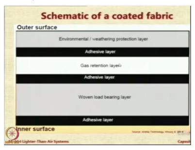
Now, today if you go to the market and look for some standard airship fabric which is used for carrying passenger carrying airships, you will find that the laminate consists of one outer layer for environmental production and weathering, that there is an adhesive, there is a layer for gas retention, then there is an adhesive and then there is a load bearing layer and then there is an adhesive layer.
