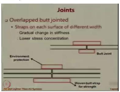
Another place which is of real concern is joints when you join the fabric together. So, how do you join fabrics together? You could do it by adhesives, you could do it by thermal welding that is by fusing the material together by heat if it is heat joinable. You could also do it by what
