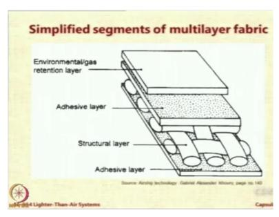
Here is a sketch of the kind of fabric which is typically used nowadays. So, you have a structural layer mostly Nylon 66 which is consisting of woven fabrics. So, because it is woven, the fabric can give you bidirectional strength and these fibers are entwined with each other in such a manner that the load is transmitted along the entire surface.
