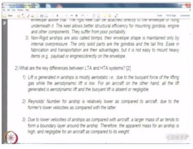
Between LTA and HTA systems, the differences are clearly mentioned in the notes. The first and foremost is about the nature of lift transition. Aerostatic lift is available in LTA systems. The Reynold's number of the airships tends to be large because of the large dimension, although the speeds are low but the dimensions are quite large. So, for an aircraft we normally had Reynold's number in terms of 6 million, 10 million.
