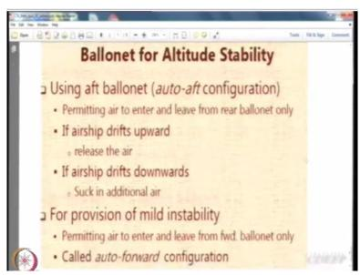
Now ballonets can be used to provide altitude stability by using the aft ballonet. So, because you can have more than one in this case two ballonets the rear ballonet alone if it is adjusted, it can be used to create the required pitching moment to trim so that is what it is.
