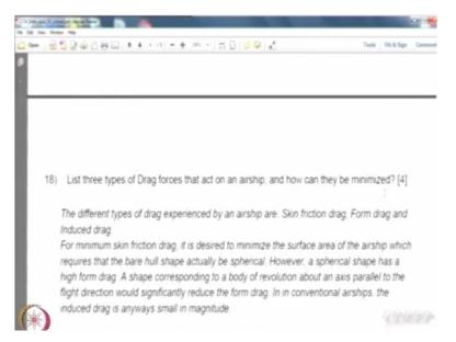
So, the three drags are skin friction form and induced. Form and profile are interchangeable. Now, for minimum skin friction drag you just try to go for minimum surface area, but spherical shape is the best for that. However, it has got extremely high form drag. So, the compromise will be an oblate spheroid type of shape. Then if you want to really worry about form drag more than skin friction, then you can go for elongating the body and making an axisymmetric body of evolution.
