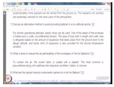
This alternative method for providing the buoyancy control, I had actually mentioned in the classroom and I actually showed you also, but did I show you a picture of this? When we operated aerostats we realized that one can, I actually mentioned just like we have a bootstrapping, you can put an elastic cable on the bottom of the envelope and you can tighten the envelope.
