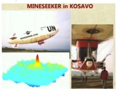
The picture on your right shows how instrumentation can be mounted on the airship for scanning for mines and the picture on the bottom left with the red peak shows you the result of scanning that was done using airship for locating the mines. The red peak indicates a return where the mine is expected to be located. So then people know where the mine is now you can send equipment to remove the mine without the need to scan the whole landscape. This is one very interesting application.
