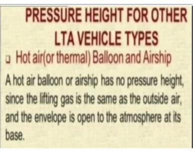
Now if you look at the hot air airship or a thermal balloon, what is there inside that? You have a chamber which has got hot air and you have a heating element below and the throat is open. There is no ballonet there. There is no pressure height because the lifting gas is the same as the outside air and it is open to the atmosphere at its base. So just by virtue of heating the air you create buoyancy.
