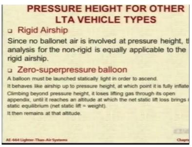
Let us look at a rigd airship. Now rigid airship does not have any ballonet. It just has gas bags inside a structure. So, the analysis that was done so far is applicable for them also. Now if you look at zero-superpressure balloon that means a balloon which is having the pressure inside just equal to atmosphere, this is called zero-superpressure balloon. Now, let us assume that this balloon, now this balloon it has to go up. It cannot have no buyoncy.
