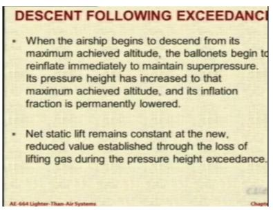
Now let us look at a situation when the airship has exceeded the pressure altitude and then it starts descending. So, this is an operational issue. There is no numerical calculation here, just observe carefully and try to understand the physics behind what is happening. So, you have reached the maximum achieved altitude and now you are descending. As you descend the ballonet will start collecting air. Why?
