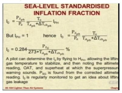
Now let us look into this little bit more deeper and see if we can get. So once again I am replacing the previous expression. I am just calling it as  $I_0$  and  $I_{PH}$  where  $I_{PH}$  stands for the inflation fraction at pressure altitude, pressure height and  $I_0$  as the inflation fraction at the sea level of the ground conditions. But  $I_{PH}=1$  because at pressure altitude the ballonet becomes flush.
