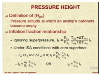
And first of all let us see if we can define pressure height and from now on we will call it as  $H_{ph}$ . So, this is the definition of pressure height about which you are all familiar. It is a height as the airship keeps climbing, we release the air from the ballonet and you reach a height at which the ballonet become flush and there is no air left in the balloon. So, that is the pressure height and the analogus definition will be the ceiling for an aircraft.
