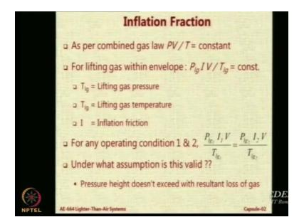
Let look at the first of these factors which is the inflation fraction I. Now applying a simple gas law which says; that PV/T is equal to constant. For any lifting gas inside a closed envelope, we can always say that  $\frac{P_{lg}IV}{T_{lg}}$  is a constant. Why do we say this because I into V is the multiplication of inflation fraction with the volume? Now in my previous slide I have used V<sub>env</sub> for the envelope volume because there is a mix up in velocity also.
