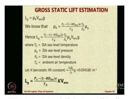
Next concept very quickly to be done is the static lift. So, the gross lift is  $\rho_A V_{env} g$ , we have already seen this and we also know with all the error in e, which I will correct when I upload this line  $\rho_A$  can be related to this number. So therefore,  $L_g$  will be just the value of  $\rho_A$  it will be that same expression into  $V_{env}g$  this is how you can calculate the gross lift. This nothing the same formula with  $V_{env}g$  added at the end of it.
