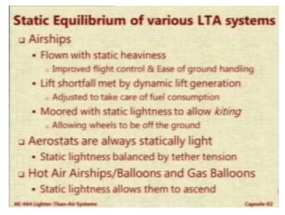
So, airships are normally flown with static heaviness okay. The reason is the flight control system is improved if you have a statically heavy system plus the ground handling is also improved. Because if a system is statically light, it will keep bubbling up. As soon as the wind comes a small lift gets generated because of the dynamic forces because it is statically light or even neutral it will start going up.
