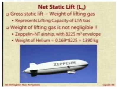
Now, the net static lift is going to be the gross static lift minus the self-weight of the lifting gas because the lifting gas will have its own mass, correct. So, this is important for us. Because this represents the lifting capacity of the gas. You may have a very large gross static lift, but if the gas where itself is very large of course it has to be less than air, but still let us say it is almost equal to air. For example, the hot air.
