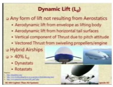
Now, although we are looking at aerostatics, we also have to understand what is dynamic lift as far as LTA systems are concerned. Now, any form of lift that is generated in an LTA system other than because of buoyancy. It could be because of the engines, by tilting the engines. It could be because of the aerodynamic force acting on the body because it is a bluff body. The bluff body when it flies at some angle of attack, it will definitely generate lift.
