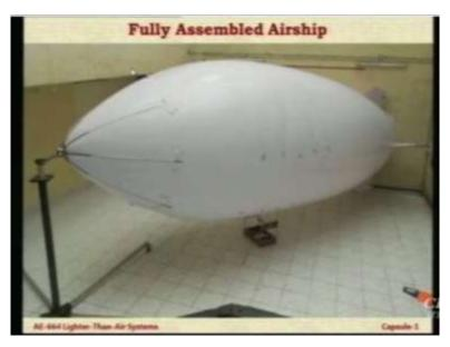
Now, let me go ahead and show you this is a picture of the assembled airship. As you can see it completely occupies the aero foyer space, there is hardly any space left. So, that gives you an idea about the dimensions This was 8 meters envelope length and the mast occupies another 3 or 4 meters because of the long legs on the other side. You can see one leg and also one more leg on that side.
