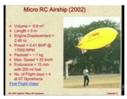
So here is the first one. The remotely controlled airship designed by the students of the 2002 passing batch. This was part of the aircraft design laboratory course, a course which is also going on right now AE 417. That year in AE 417 since I was completely occupied with airship and airship research, I requested the students why do not they work with me in developing an airship.
