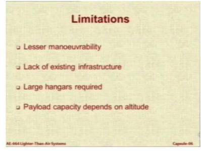
So, these are the four basic limitations of the cargo airships. First of all, they will not be as maneuverable as aircraft because they are bulky in shape and because they are buoyant body. And secondly, their large size will require totally new infrastructure. It is very difficult to expect that you make these airships and you can operate them from existing cargo hangars because existing hangars are not so large in size.
