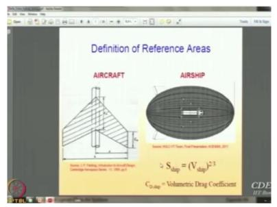
So, this is what we have already seen in the last couple of minutes. For aircraft, we have this cross sectional area including the, not cross sectional area reference area including the area inside the fuselage. And for the airship we have  $Volume^{2/3}$ .
