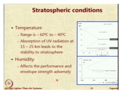
So, move on. So, the temperature range is -60 to -40 degree and that will affect envelope as well as it will affect the buoyancy, it will affect the power output from solar cells. Humidity is there. At that height humidity is less because humidity creates always a problem. It decrease the strength.
