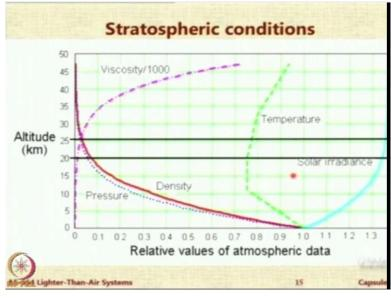
So, let us see what are the actual scenario at that height. So, at the altitude of around 20-25 kilometers, you will see the temperature and density and viscosity at that range it is actually optimum. You do not want to have very low low density because it will affect our buoyancy as well as if you will place below that height, higher density will lead drag and the temperature and solar irradiance. So, at that particular height it is optimum.
