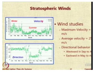
So the wind profile. It is actual wind studies shows the variation of wind over the year and goes a maximum up to around 45 to 50 meter per second and average velocity of 25. And actually the wind velocity and its direction is a major problem because when direction changes, you have to optimize the orientation of airship to minimize the drag because same wind velocity and airship is in longitudinal direction and lateral direction the drag will be different.
