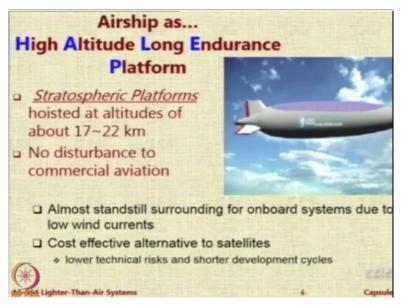
So high altitude long endurance platform. Long endurance basically is for because it can stay at that height for a couple of months, 6 months, may be for even a year. That is why it is called a high altitude long endurance platform. And it remains a standard still and serves the purpose as standstill platform. And it is very cost effective relative to the satellite because designing and launching and sending at that height is very cost effective relative to the satellite.
