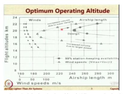
So, why question arises why it is placed only at 20 or 25 kilometers that is why it is answered here. So, the wind speed at that height is relatively lower. Below that due to the higher wind speed, so at high wind speed to overcome that drag because this system used to have very big and to overcome that drag you will need bulky power systems to overcome that drag. Otherwise, it will shift to another location.
