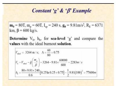
So let us consider the same problem that we had considered for ideal burnout solution that we have a liftoff mass of 80 tons, the propellant mass of 60 tons, same  $I_{sp}$  of 240 seconds and the sea level gravity of 9.81 and we introduce two parameters which we are going to additionally need. One the burn rate  $\beta$  and currently it is chosen as, these may be arbitrary number of 600 kg/s just to understand the implication.
