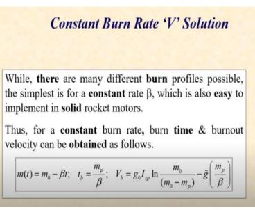
Of course, as we have already seen, there are many such possibilities that one can think of for burn profiles. But the simplest that we can at this point make use of is the constant rate  $\beta$  which indicates that the propellant burns at a constant mass flow rate which is also easy to implement in solid rocket motors. In fact, you will find that by and large solid rocket motors burn at a constant rate of burn.
