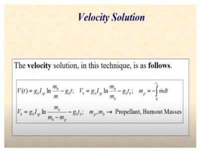
Let us now extract the velocity solution through this technique. And we find that it is now a simple matter to perform integration of the differential equation given by  $\frac{dv}{dt} = -\frac{\dot{m}}{m}g_0I_{sp} - g_0$ . So, when we integrate the differential equation, the first term is same as what we have obtained for the ideal burnout case.
