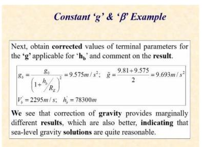
One way, there are number of ways of course one can do that, but one way of doing this is to use a value of an average gravitational acceleration between the sea level and the 78 km point. We can use a simple arithmetic average and see in what manner our solution changes. Let us see what is the implication of such a hypothesis of using an approximate gravitational value, which is an average of the gravitational value at sea level and 78 km altitude.
