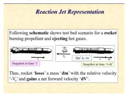
So let us look at this particular representation of a rocket engine firing. So, consider the following schematic in which a rocket is burning propellant and ejecting hot gases. Of course, in this case, we have introduced a velocity vector V just to make the derivation more general. But we could very easily make this velocity equal to zero which would represent the test bed configuration.
