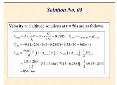
So let us first obtain the velocity at altitude solutions at t = 50s. So, at t = 50s the amount of propellant that we are going to consume will be given by, because it is a constant burning rate, I know that I will burn all the propellant in 156 seconds. So, in 56 seconds, I would be burning only a small amount of propellant. So, propellant burned ratio becomes only 0.2885.
