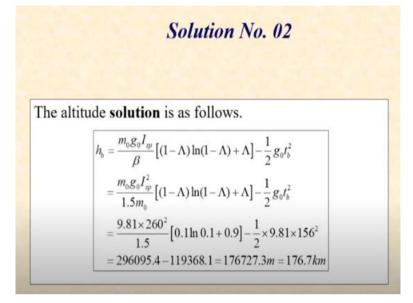
So, in this case, we recall the altitude expression which is  $\frac{m_0 g_0 I_{sp}}{\beta} [(1 - \lambda) \ln(1 - \lambda + \lambda)] - \frac{1}{2} g_0 t_b^2$ . Now as  $\beta$  is a function of  $I_{sp}$  and  $m_0$ , I substitute that  $\frac{1.5m_0}{I_{sp}}$ .  $m_0$  will cancel. And what will be left will be  $\frac{g_0 I_{sp}^2}{1.5}$ .  $\lambda$  is already specified as 0.9. So, this will become 0.1 ln 0.1 + 0.9.
