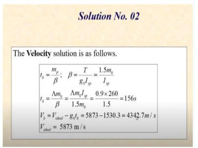
So, the velocity solution is as your burnout time is nothing but the ratio of  $\frac{m_p}{\beta}$ . And please note, we have not specified the  $\beta$ , what we have specified indirectly is the lift-off thrust which remains constant. So, which means we have specified thrust and from thrust we must discover the burn rate  $\dot{m}$ . So, we bring in that idea. So  $\beta$  is nothing but our  $\dot{m}$  and that is nothing but thrust divided by  $g_0 I_{sp}$ .
