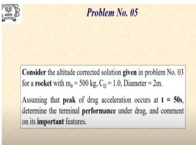
So let us consider the altitude corrected solution given in problem number 3. So, in problem number 3, we have corrected the altitude because of the change in gravity. And that is the new gravity value is what we have used for terminal velocity. So, we have a velocity of 4380 odd m/s and the altitude of almost 180 km that is 179 odd km.
