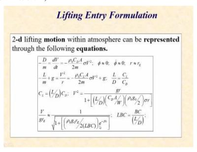
As the trajectory is primarily a two-dimensional motion, this motion can be represented in atmosphere through the following equations. So again, we have the same set of equations for the equation in the direction of velocity that we have already seen for our ballistic entry with specific assumptions that the flight path angle is nearly 0.
