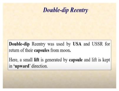
In contrast to the skip reentry, the double dip reentry was used by USA and USSR for return of their capsules from the moon when they were synthesizing the Apollo missions and similar moon missions. In this case, we generate a small lift by the capsule, there was no wings basically. So, this lift is actually quite small. And typically, initially it is kept in upward direction.
