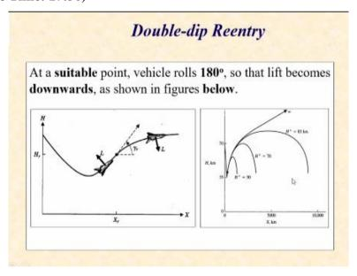
At a suitable point based on the requirements of the trajectory, the vehicle is allowed to roll by 180° without making any other changes to its altitude, so that the lift vector flips by 180° and it acts downwards along with the weight as shown in the picture below.
