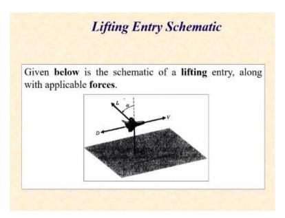
Given below is a schematic of a lifting entry along with the various forces that act on the vehicle during this phase. So, you have an aircraft like vehicle that has a velocity V and has a drag which is opposite to the velocity vector and we have a lift which is normal to the velocity vector. In addition, the weight acts along the downward direction or the gravitational direction.
