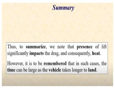
Thus, to summarize, we note that presence of lift significantly impacts the drag and consequently the heat. However, we should also note that in such cases, the time can be large as the vehicle takes longer to land. Hi, so in this lecture, we have seen the use of lift vector to arrive at different types of reentry trajectories to manage the heat load and the deceleration of the vehicle.
