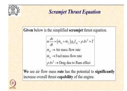
So given below is the simplified Scramjet thrust equation. And you will find that this is similar to the thrust equation that we had seen in the context of a conventional rocket except for one important difference which makes the Scramjet engine generate lot more thrust. As you can see,  $\dot{m}_{in}$  is the air mass flow rate while  $\dot{m}_f$  is the fuel flow rate. So, in the conventional rocket, the thrust is  $\dot{m}g_0I_{sp}$ , which is  $\dot{m}_f$ .
