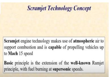
The Scramjet technology essentially makes use of atmospheric air to support combustion and is capable of propelling vehicles up to Mach 15 speed, which means that we can achieve very high speeds which is a requirement for sending the objects deeper into the space.
