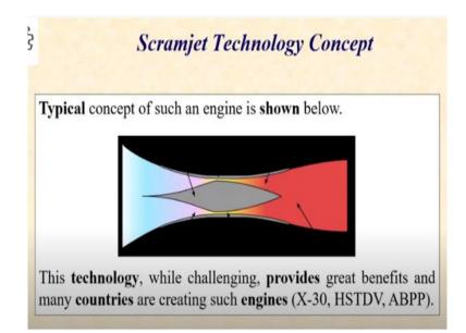
Typical concept of such an engine is shown below. So, this is a typical sketch of a Scramjet engine which takes in the air coming at hypersonic speeds that is speeds well beyond Mach 4 or 5. Then creates a supersonic diffuser of using cross sectional area that significantly increases the pressure until it reaches a very high value.
